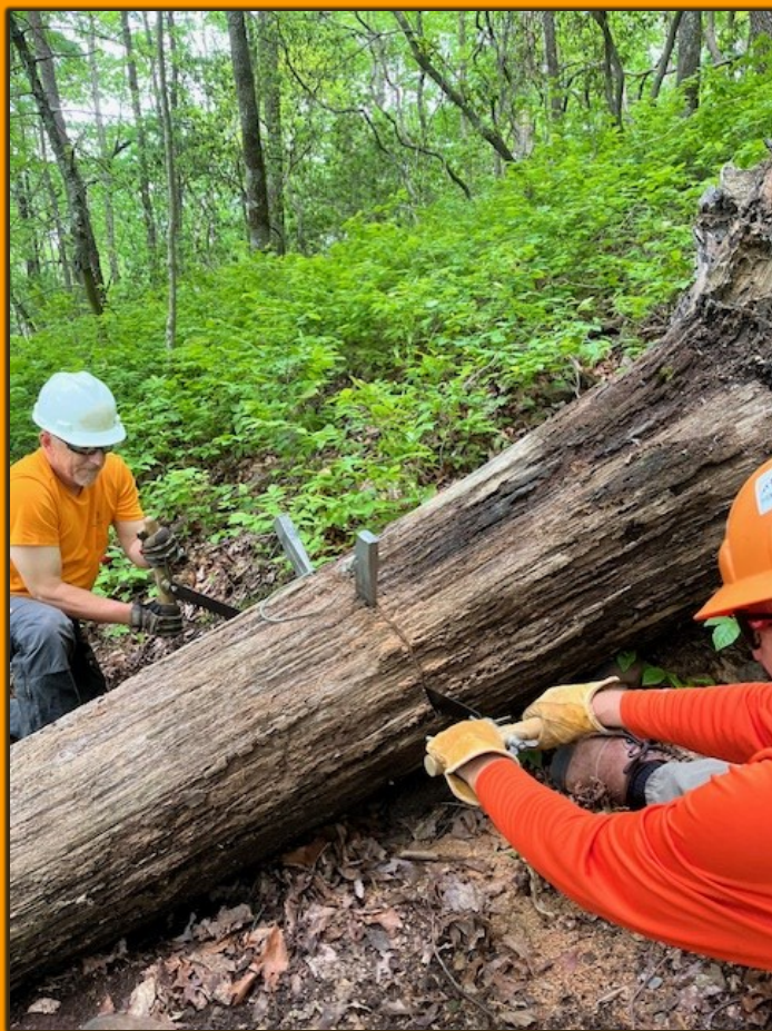
Brian Trinkle and Ed Sullivan muscling the crosscut saw. Note the use of wedging to aid in an easier saw.
